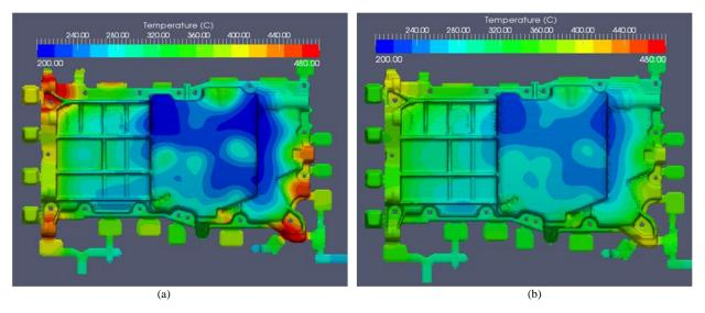
Fig.5. (a) Casting temperature before optimization, (b) Casting temperature after optimization
