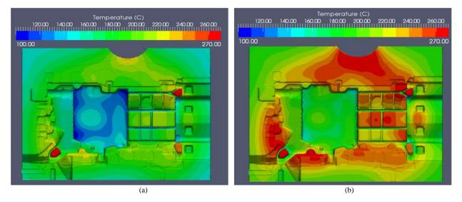
Fig .6. (a) Mould temperature before optimization, (b) Mould temperature after optimization
